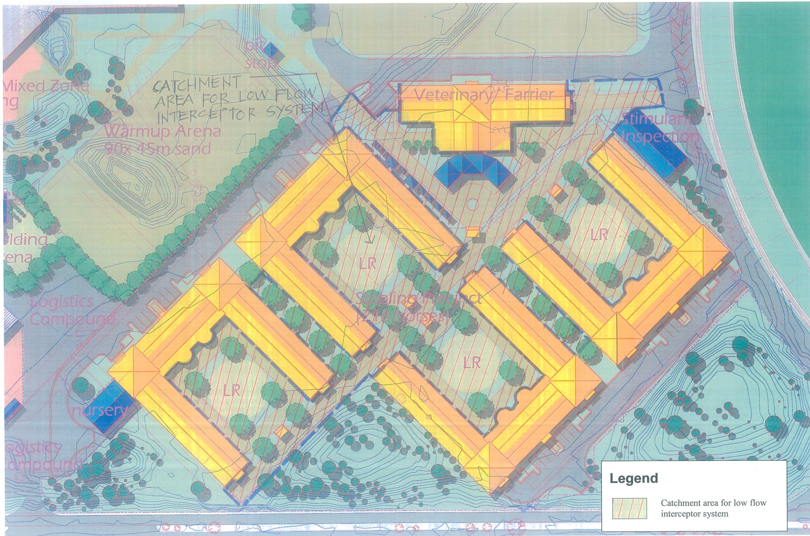
Proposed Catchment Area for Low Flow Interceptor System – Hong Kong Sport Institute Site
